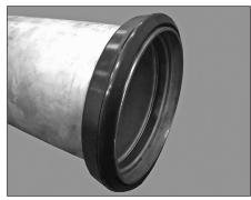
**3. POSITION GASKET:** Position the gasket over the pipe end. Make sure the gasket does not overhang the pipe end.
