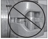
9. Inspect the bolt pads at each joint to ensure proper assembly is achieved (gaps are equal at each bolt pad and the required torque values are achieved).
