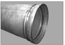
1. CHECK PIPE ENDS: The outside surface of the pipe ends must be smooth and free from indentations and projections to ensure a leak-tight seal. All oil, grease, and dirt must be removed.
